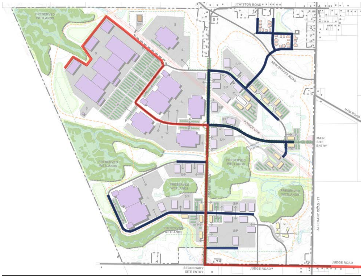
FIGURE 2: Phase 1 natural gas service is shown as a red line, while extension of the system to accommodate build-out is shown in the blue lines.
