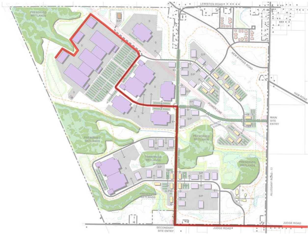
FIGURE 3: STAMP Phase 1 Natural Gas system
